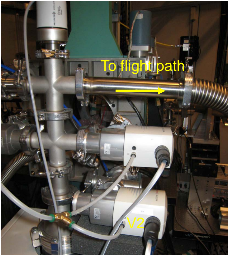
Before: V2 unconnected, hose to flight path connected without valve
