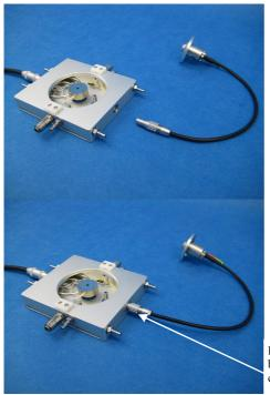
Pull the connector shell backwards to release the cable assembly
