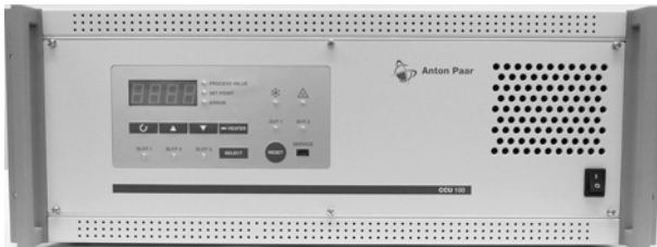
Fig. 6-1: Front panel of CCU 100
