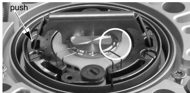
Fig. 22: Mounting of the ASS
