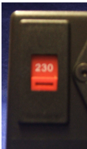
Fig. 5A – AC Line Voltage Select switch position for 230V operation
