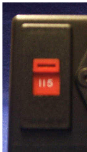
Fig. 5B – AC Line Voltage Select switch position for 115V operation
