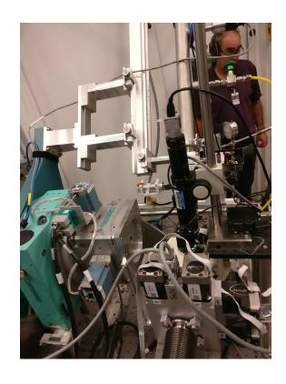
Microscope was placed above cryostat quartz window using posts and the sample was imaged for 10 hours at 78K. Results are displayed on next page
