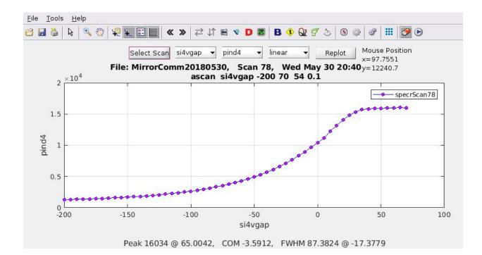
Try si3 as the beam defining slit, parasitic clean up with si4 and si5 seems good, both silicon soft slits
