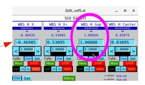
8ida:Slit1Hsize.VAL 2019-2 standard conditions: For 7.35 keV = 0.04 (2D focus) For 10.9 keV = 1.00 mm
