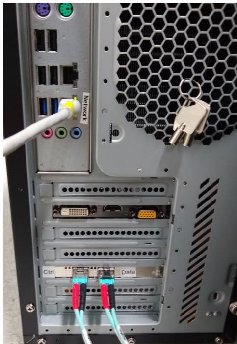
Figure 6: Connections on back of control PC
