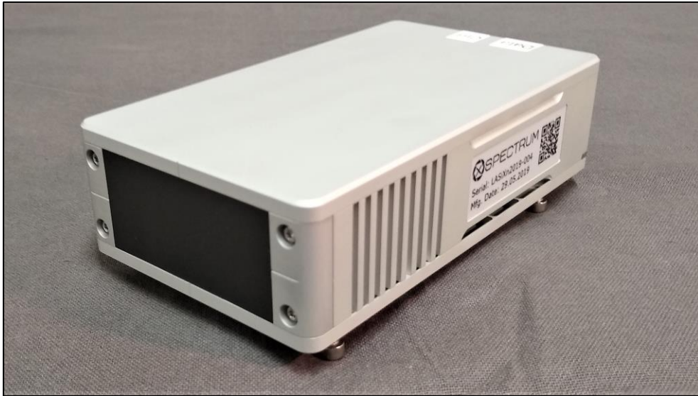
Figure 1: The Lambda detector. The black region is the carbon fibre cover.
