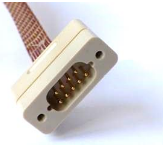
Figure 1 View of output wire of the mechanism with a Male Sub-D 9 connector (High Vacuum compatible).
