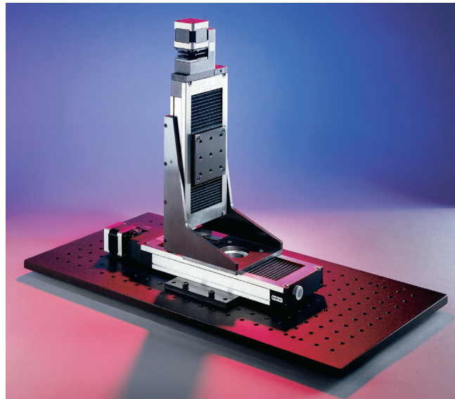
(M-)UTM X-Z assemblies can be aligned to within 50 \mu rad orthogonality and can provide up to 150 mm of travel.
