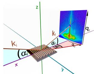
$$q_{x,y,z} = \frac{2\pi}{\lambda} \begin{bmatrix} \cos(\alpha_f)\cos(2\theta_f) - \cos(\alpha_i) \\ \cos(\alpha_f)\sin(2\theta_f) \\ \sin(\alpha_f) + \sin(\alpha_i) \end{bmatrix}$$
